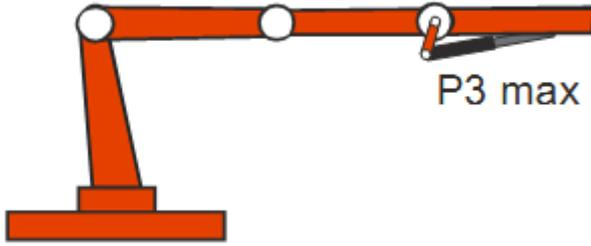
If the crane has a JIB, the booms are extended as above. When fully extended, the permissible load is lifted and the pressure P3 read from the display at the same time is set as the limit pressure.
