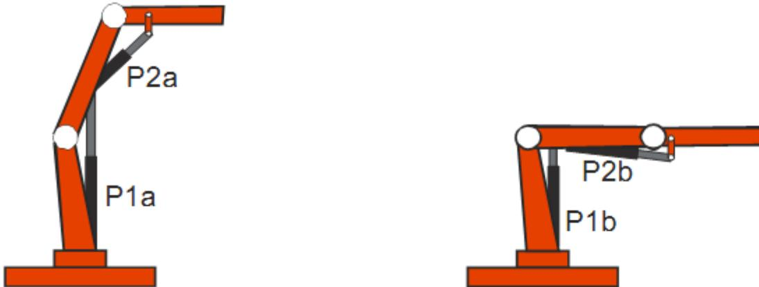
For pressure calibration, the maximum pressure on the Main Boom (P1) and Knuckle Boom (P2) cylinders must be read from the display. Therefore, the booms are moved to each of the 2 positions above and are extended so that the load chart permits. The permissible load quantity is lifted and the pressure values are measured in the load chart.
